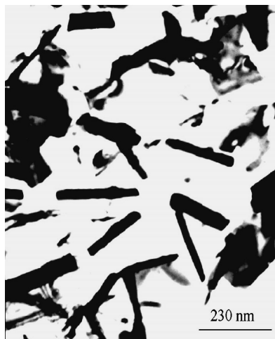
Figure 2. TEM image of the SnS nanorods obtained after 2 h reaction time.
